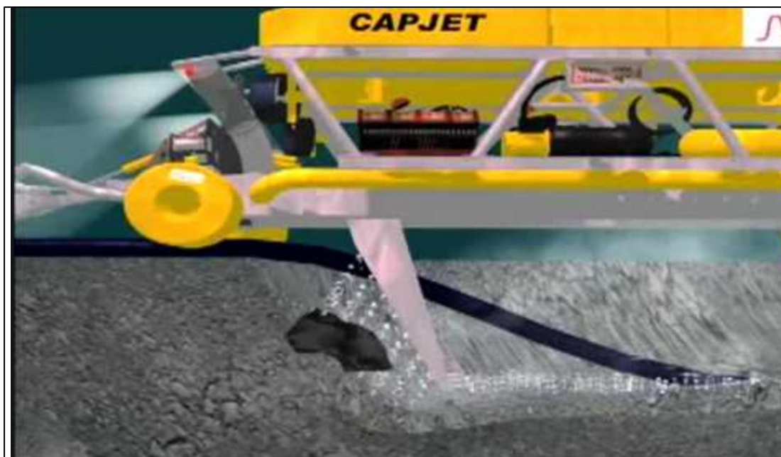
Figure 4.1: Nexans CAPJET Burial Tool.
